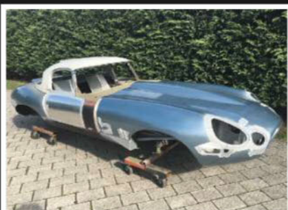
JAGUAR E TYPE. Lightweight steel monocoque, all Ali out panels £POA
